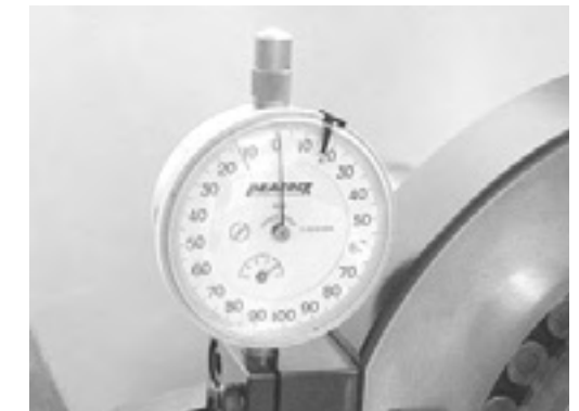
Fig. 1.15 Measurement of Spacer Width
