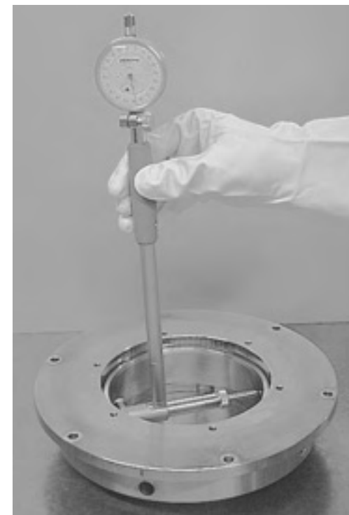
Fig. 1.10 Zero Setting of Cylinder Gauge
