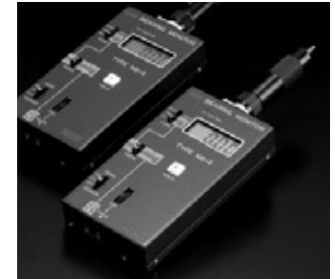
Vibration Measuring Equipment, Bearing Monitor NB-4 (See Page 128)
