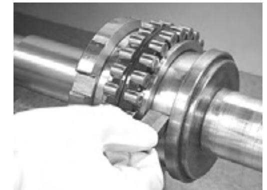
Fig. 1.15 Measurement of Spacer Width
